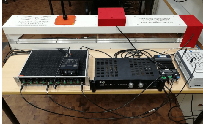
(a) A Photograph of the experimental setup with the duct placed behind the used filter, amplifier, signal generator and the hardware platform. [Han+18]
