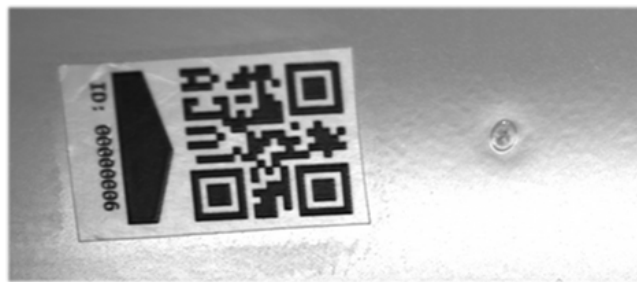
Figure 2: Positioning an annotation sticker near an anomaly
