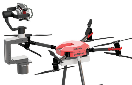
FIGURE 3. Rendering of the developed UAS with the C-shaped sensor-mounting
