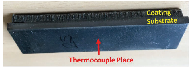
FIGURES 1: PLACEMENT OF THERMOCOUPLE FROM THE BACKSIDE OF THE SUBSTRATE. A DEPTH OF APPROX. 2 MM, APPROXIMATELY REFERS TO A DISTANCE OF 1MM TO THE SUBSTRATE SURFACE
