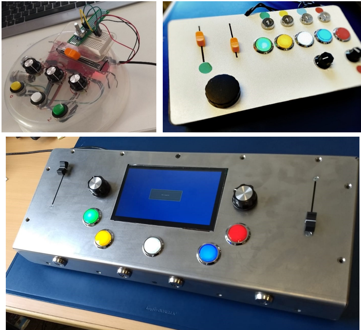
Figure 6. Different stages of hardware development for the response box.
