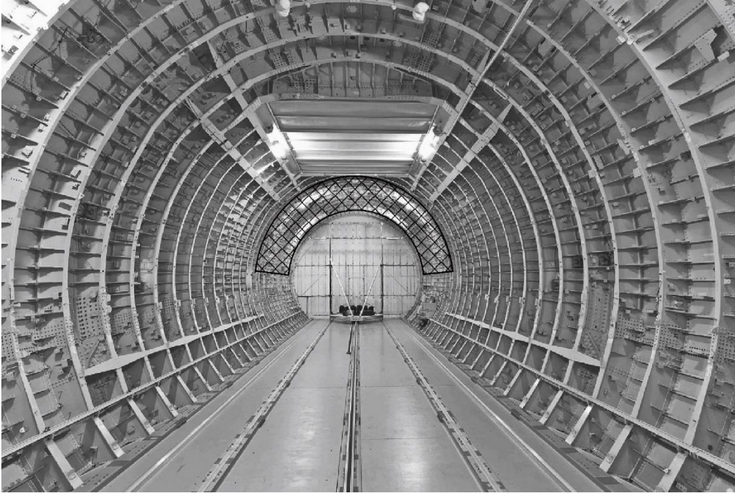
FIG. 8. Photograph of the fuselage interior with a microphone measurement frame in the back, wooden floor panels on the ground and rubber mats covering the central wing box. The sector of measurements with the LDV is cross-hatched.
