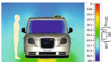
Fig. 1. Example of a person exposed to a stray magnetic field from a WPT system in the TALAKO project ( https://talako.uni-due.de/ )
